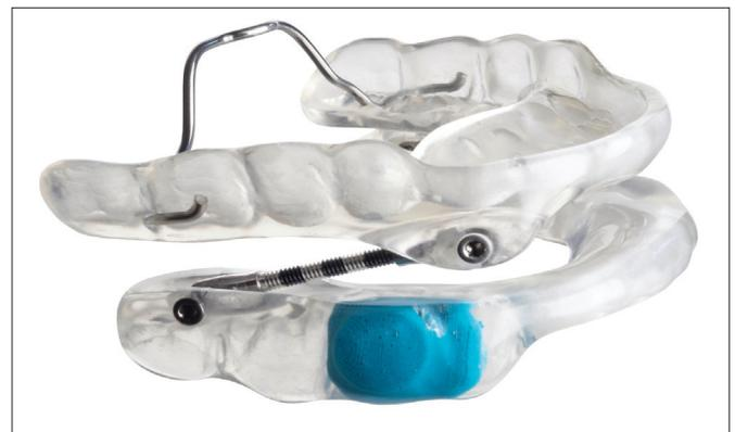
**Figure 1.** The Protrusor® MAD device. It is made of two resin splints connected by two threaded titanium bars, which can be regulated to reach the desired amount of mandibular advancement. A chip for compliance monitoring is embedded in the lower resin splint.
